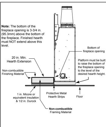
Figure 12.3 Raised Platform Hearth Extension Detail
